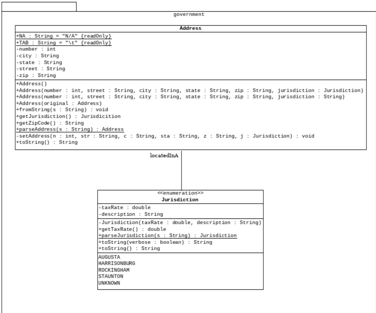
In addition to the specifications that are contained in this class diagram, the implementation must comply with the following specifications.
