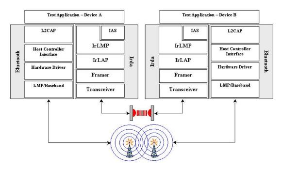
Figure 2. Bluetooth and IrDA Stack Diagram
