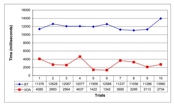
Figure 9. Device Discovery and Connection Establishment.
