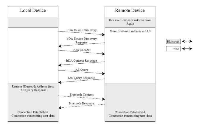
Figure 5. IrDA-Assisted Bluetooth Connection Procedure
